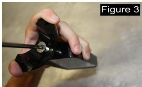
Step 4: Continue holding the two pieces and install supplied Allen head bolt to secure the two pieces. Repeat steps 2 & 3 for the other side of UTV.
