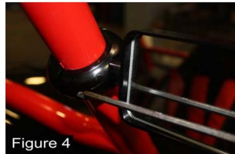
**Note:** *Clamp may scratch cage when installed*
