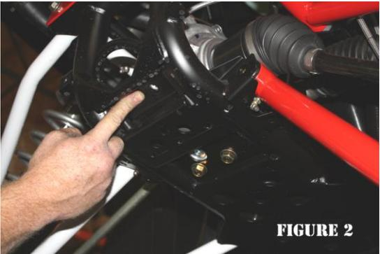
**Step 5:** Using two (15mm Wrenches) remove lower A-Arm retaining bolts.
