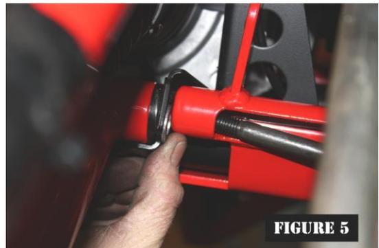
**Step 10:** Remove two lower bolts on front grill frame and loosen two upper bolts using (13mm Wrench) swing upwards and out of the way. Tighten upper two bolts to secure into place temporarily.
