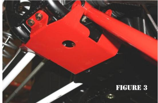
**Step 7:** Install lower A-Arm rear mount gusset plate **(B)** and be sure to feed plate **(B)** under throttle cable **(See Figure 4)**
