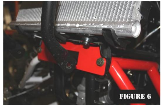
**Step 12:** Slide upper A-Arm rear gusset plate (F) onto factory bolt and secure with new supplied nut (G) finger tight. Then bolt it to lower gusset plate with supplied hardware (H) using (2) 9/16 Wrenches) (See Figure 7)
