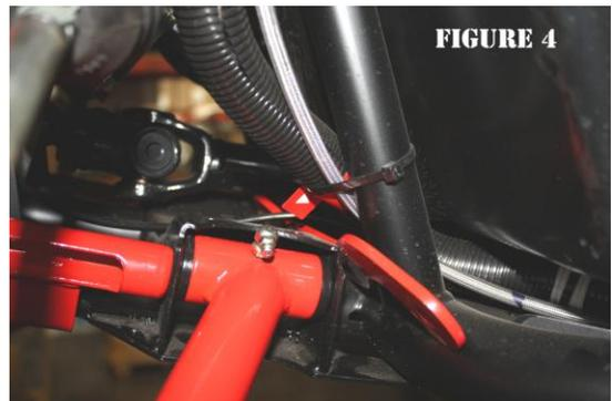
**Step 8:** Install new supplied hardware **(C)** for lower rear A-Arm mount through rear lower gusset plate and rear mount gusset plate, finger tighten.
