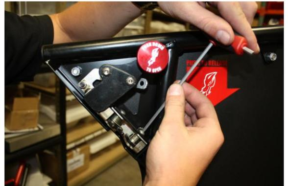
**Step 12:** Now you will need to set the lash of the door handle to preferred amount. To achieve, loosen the set screw on top of latch lever with 2mm Allen wrench. Adjust by threading parallel brass set screw in or out using 2mm Allen wrench. Check operation of door latch, some lash may be required for smooth operation. Once proper lash has been reached re-tighten set screw on top of latch lever. (**As seen right**)
