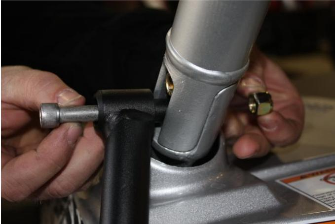
**Step 7:** Place frame up to car. Starting at the front, install supplied Allen head bolt through front mount of door frame and into stock location of lower cage bung bolt with 5/16 Allen wrench. Secure using stock nut retained in previous step; finger tighten nut (be sure to allow enough play so that frame can be raised and lowered). (**As seen left**)
