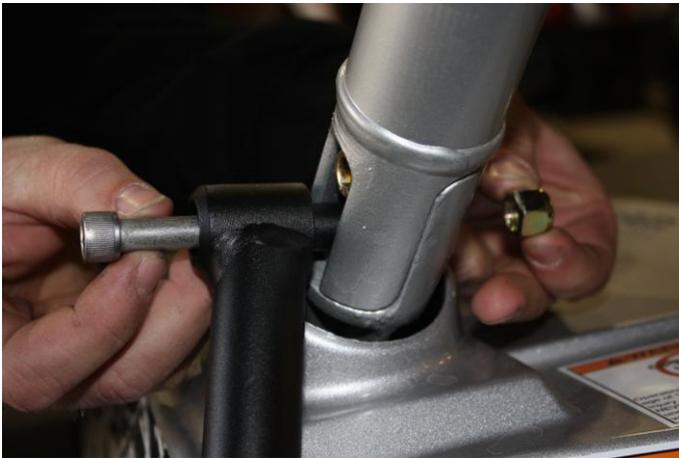
**Step 8: Lower door frame down to resting position. Center rocker hook should be completely over rocker. Rear door frame mount should now fall on top of stock B-Pillar cage mount. Re-install stock bolt and nut with 17mm or 13mm wrench & Socket depending on year, through both rear door frame mount and B-Pillar cage mount; finger tighten. (As seen below)**
