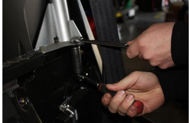
**Step 7: Place frame up to car. Starting at the front, install supplied Allen head bolt through front mount of door frame and into stock location of lower cage bung bolt with 5/16 Allen wrench. Secure using stock nut retained in previous step; finger tighten nut (be sure to allow enough play so that frame can be raised and lowered). (As seen below)**
