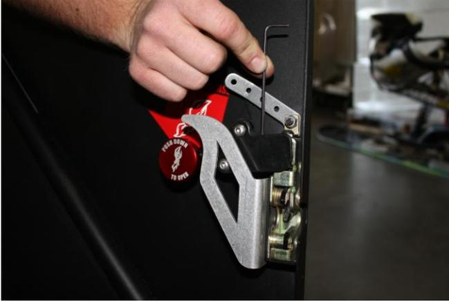
**Step 13: Test the function of the door. Open and close door as well as familiarize yourself with the locking mechanism located on the top of the latch (note door will not open or close when locking lever is engaged). To lock door latch depress lock lever downward to unlock door latch lift lock lever upwards.**
