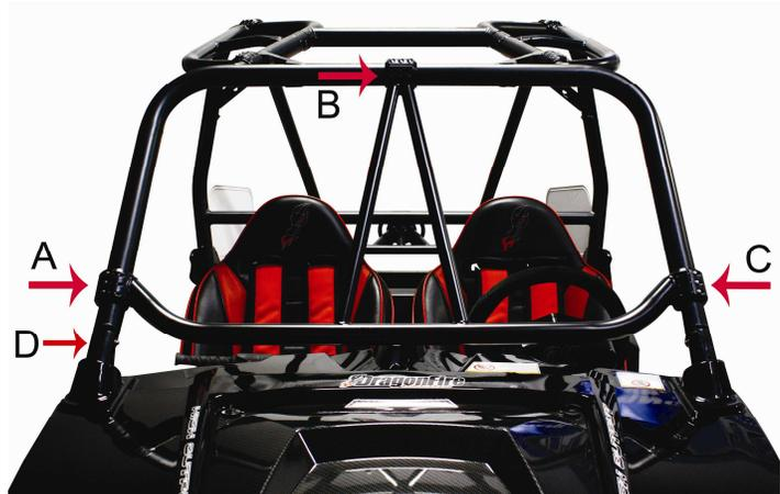
**Step 4:** Place Flying-V inside front portion of cage, check to see that all cage clamps are sitting flush against cage. Loosely re-install top piece and all six bolts to cage clamp **(B)**.
