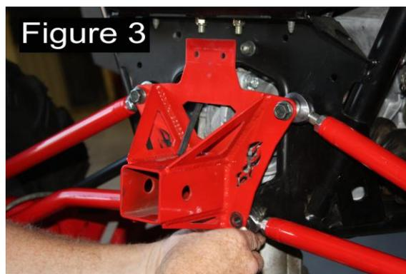
Step 5: We recommend you evenly tighten each bolt to 50 foot pounds using torque wrench. If you do not have access to a torque wrench evenly tighten hand tight using socket and wrench. Install is now complete.
