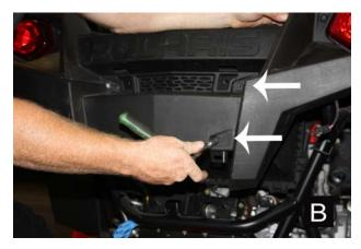
**Step 4:** Hold complete assembly up to the car and secure using hardware retained in step 3. It is best to start at the top and finish at the bottom. (See figure C)
