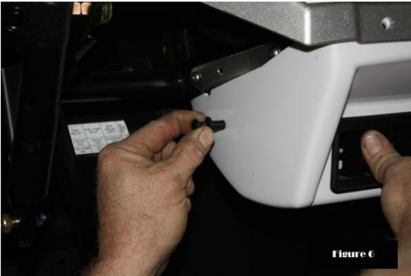
**Step 7: Secure sides of Pod with stock plastic pins that were removed in (Step 2)**
