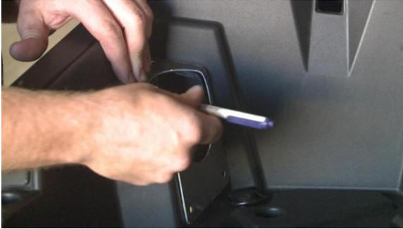
**Step 9:** Install the Aluminum hose trim cover. Align the cover over the “hump” in the rear driver side of the bed and hold in place while using a marker or pen to trace the hole for trimming. *(as seen on the left)*
