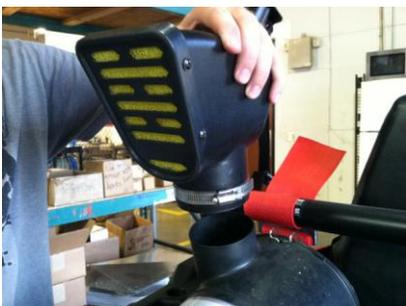
**Step 29:** Install the supplied hose clamp over the scoop base.
