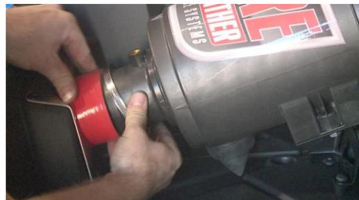
**Step 28:** Now it's time to install the intake scoop. Orientation of this scoop is a personal preference. (We typically face the scoop backwards)
