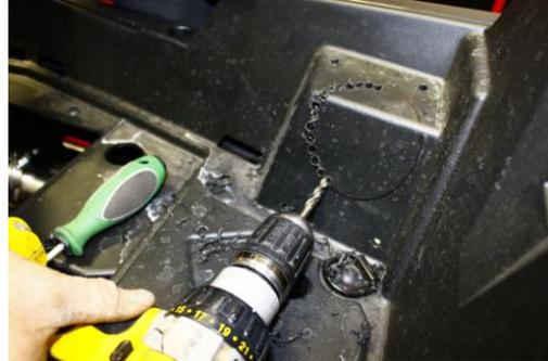
**Step 11:** Using a Razor knife cut between the holes to cutout the circle. This will leave a “saw tooth edge”. To remove this, use the razor blade or a Rotary cutting Tool to remove each “tooth” until you have a clean circle cut out.
