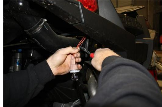
**Step 21:** To install alternative light socket you will need to remove stock tail light socket from harness
