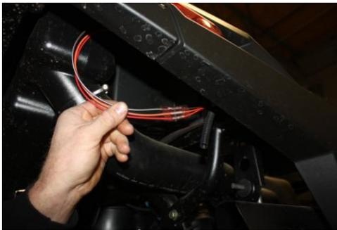
**Step 23:** Remove factory bulb from the stock light socket and insert into new 90-degree socket.
