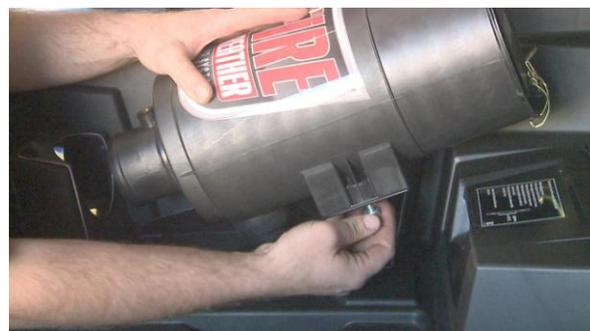
**Step 19:** Now mount the intake can to the supplied metal bracket using two 8mm bolts and washers. *(as seen above)*
